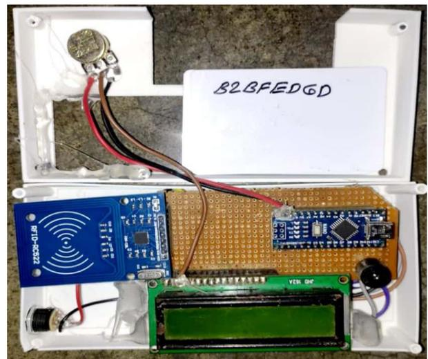
Fig -6 Actual Experimental Set-up
