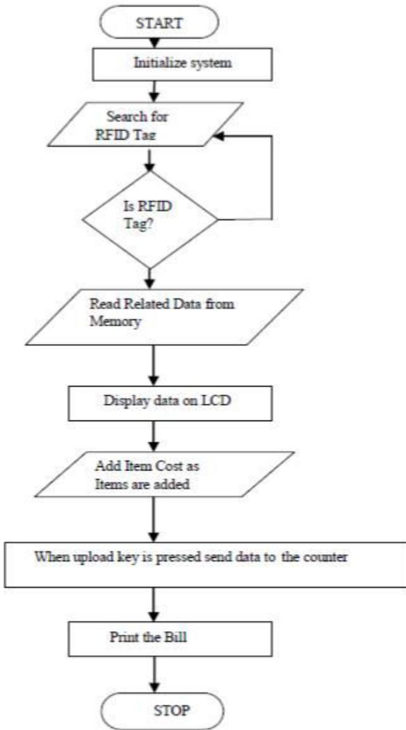
Fig -7 Flowchart of Set-up
